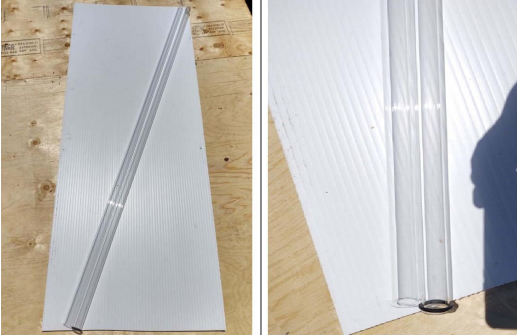
Figure 7-2: UV Lamp Fouling Sleeve Comparison: Sleeve with Black O-ring was Used in Pilot Study
